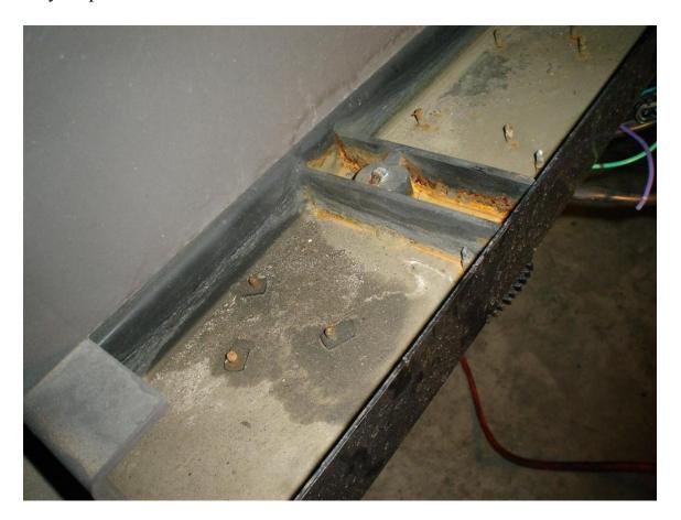
What can you do when presented with this type of mess? If nothing is done the step mounting assembly is are going to rust out, then what do you do? My first order of business was to clean up the mess, get rid of the rust and collected debris then drill two 3/8 inch drain holes in each of the three pans which had been accumulating water, dirt and anything else kicked up.
