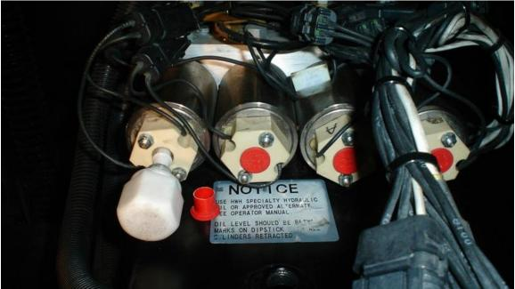
For demonstration purposes the protective cap was removed then the tank plug/nut driver was inserted over the nut in the solenoid. Again on this specific type of solenoid, the nut is **ONLY TURNED ONE FULL TURN COUNTER-CLOCK WISE** which will allow the hydraulic fluid to flow back into the tank which in turn will allow the jack to be retracted by spring pressure. The selected jack solenoid for demonstration purposes was the RR (right rear) jack.
