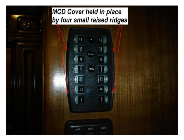
The 14 Channel remote control cover can be removed by carefully slipping a small straight blade screwdriver between the cover and the back at four access points located on the side of the cover near the raised ridges.
