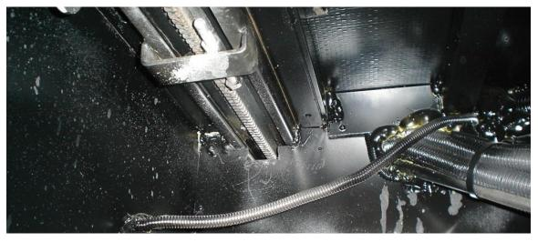
The enclosed portion of the slide mechanism and cable entry/exit was covered in a previous modification (Modification # 24) to the house battery compartment.
