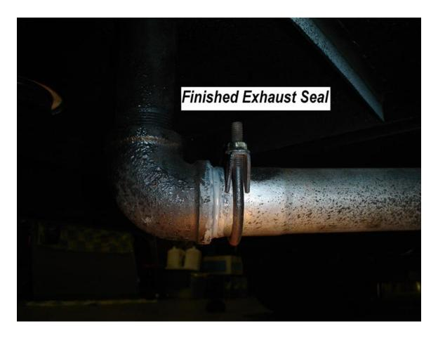
Both pipe clamps were re-installed and tightened. After allowing the sealer to cure the Aqua Hot system was again turned on and checked for exhaust leaks.
