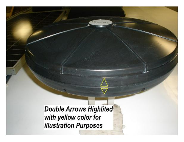
As seen in the picture above for illustration purposes the double arrows were highlighted in yellow to make the double arrow location easier to find. When the remotes button is held to the left when the antenna reaches its left limit (stop) a light will be displayed (end of rotation). Likewise when the button is held to the right when the antenna reaches the limit/stop the end of rotation light will again illuminate.
