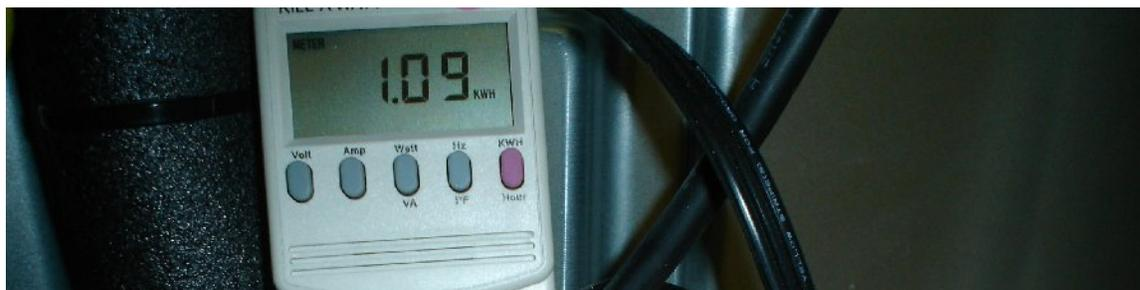
1.09 KWH's were consumed over a 20 hour and 31 minute period using my P3 Kill-A-Watt meter.
