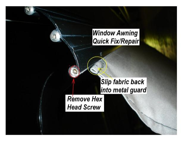
Remove the hex screw push the fabric loop back into the metal cover insert a piece of 3/16 inch dowel (cut the dowel length to fit inside the fabric loop) reinstall the hex screw and the repair has been completed.
