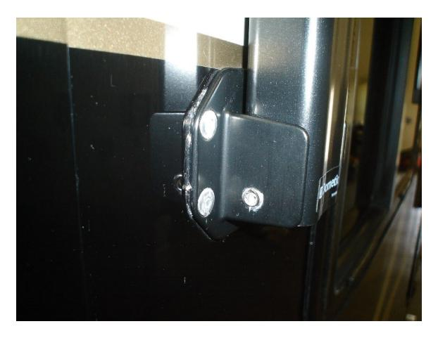
After sanding and sealing every pop rivet pin which needed sanding, attention was focused on applying silicone sealant over the head of every pop rivet.
