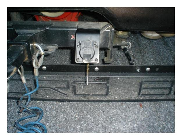
It is hoped the small 1/8 inch drain hole will prevent water accumulation in the future. If the hole does not take care of the problem, I will consider bending the OEM 45 degree mounting bracket down to a 90 degree angle which should keep the water from entering or collecting in the socket.
