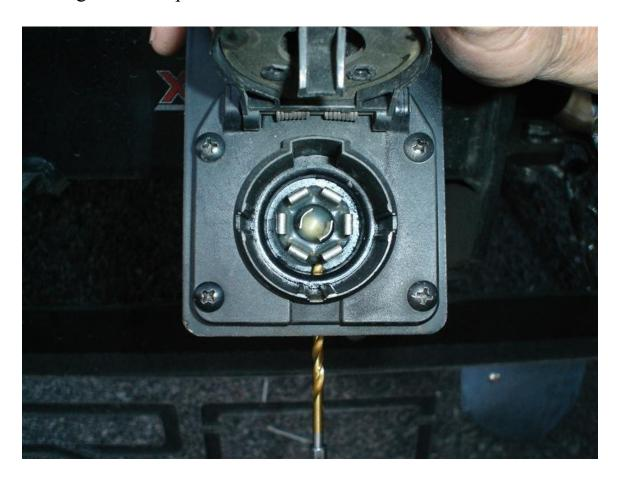
After thinking about the problem I decided preventing ANY water from getting into the socket was most likely impossible, however if I drilled a hole and allowed the water to drain out, then the water that did seep in would just pass through and should not cause a problem.
