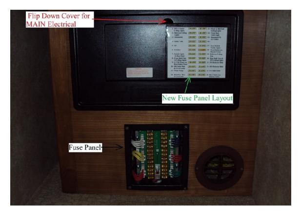
Many of Tiffin's newer model diesel coaches have the AC electrical panel and the DC fuse panels located either under the adsorption refrigerator (Norcold or Dometic) or near the rear closet. To make labeling the electrical and fuse panels easier to understand the included photos were modified to better explain the function of the individual circuit breakers or fuses.
